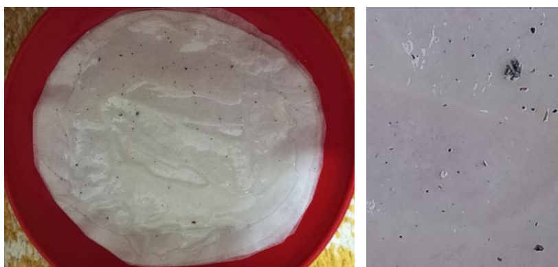
Figure 2. Macroresults from the experiment placed in Skopje (left), microanalysis of the air pollutants using mobile phone's camera (right).
