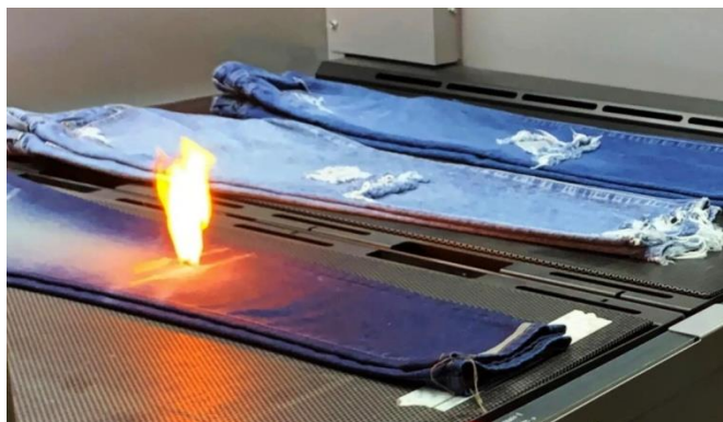
Figure 4. Small flashes of flame creating serious material damages and holes by high power laser beam https://www.cnb.com/video/2018/03/02/levis-is-replacing-workers-with-lasers-to-distress-jeans.html
