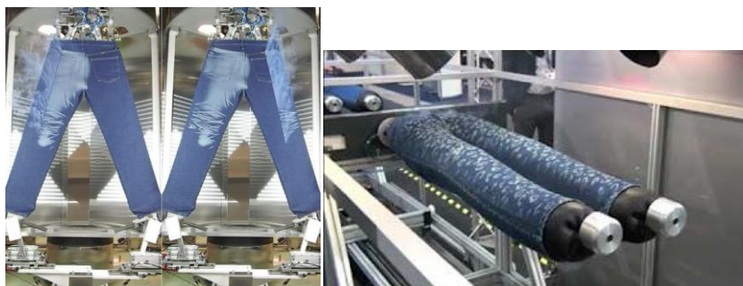
Figure 2. Mannequins fixed in horizontal or vertical position to perform denim marking by laser [14]
