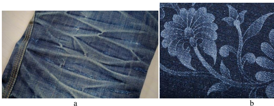
Figure 5. Honeycombs on jeans (a) and fine patterns (b) created by laser [14] https://denimhunters.com/denim-wiki/jeans-anatomy/honeycombs/
